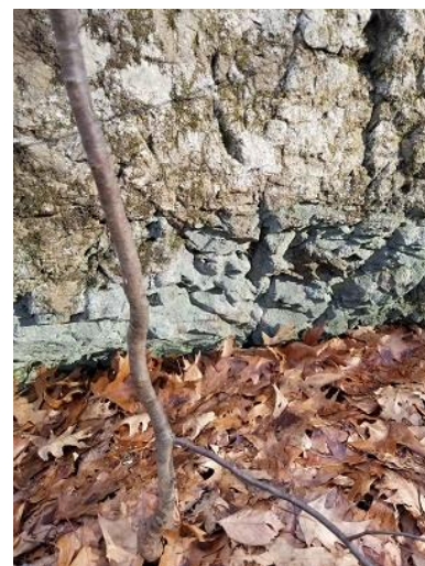
Fig 10: Weathered Dedham Granite takes on mint toothpaste tones. This color is most prominent near the leaf litter, indicating that moisture might play a big roll in the chemical process.
